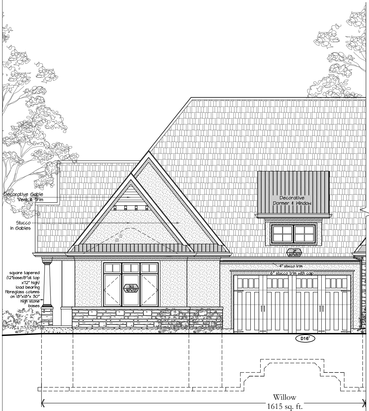
Willow Front Elevation scale: \frac{1}{8}"=1'-0"
